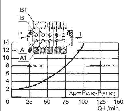
**$\Delta p$  (2 Valves in connected in series)**
